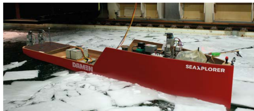
At the Hamburg Ship Model Basin (HSVA), we put the SeaXplorer to the test. The design successfully proved its icebreaking performance through extensive testing in conditions such as level ice and broken ice, including manoeuvring in ice conditions.
